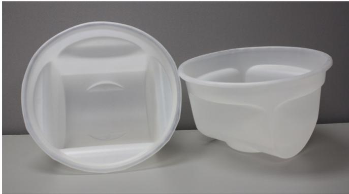
The Topliner Cradle allows you to put two different substances in a single standard 5-gallon pail. The liner has a molded lip which hooks over the top chime of the pail. The cradle is suspended over the contents of the bottom portion of the pail, separating them by a barrier of high density polyethylene.
